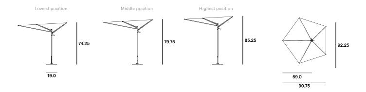
In combination with standard parasol base Height adjusting knob in highest hole
