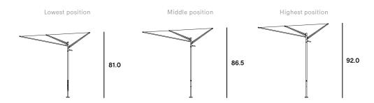
The Acacia is available in one dimension In combination with standard parasol base Height adjusting knob in lowest hole
