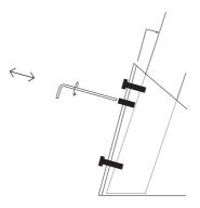
The parasol pole can be slightly tilted by turning the two adjusting screws in the two remaining holes
