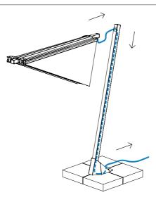
In case of optional light, insert the cable in the hole in the parasol pole and lower it down until it appears at the bottom
