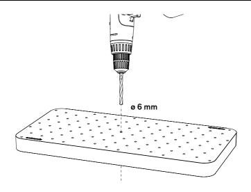
Drill a ø6 mm hole through the center of the base
