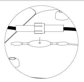
In case of Led, push all the cables deep into the recesses
