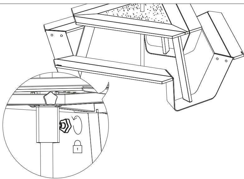
**Tighten the bolts & lock the parasol**
