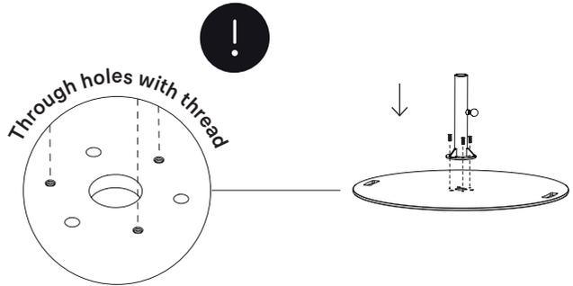
1. Place the galvanised steel base plate on the ground and mount the stainless steel tube on it with 3 bolts M6x12. Attention: Make sure that you fix the bolts in the thread of the base plate as shown on the drawing.
